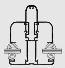
PR 100 is a non-insulated aluminium roof system that can be used as a terrace covering or a carport. PR 100 offers a range of rafters in different heights and widths so that high static requirements coming from snow load and own weight can be implemented without using steel reinforcements.
